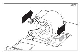
■ Plug the connection cable from the ventilation system into the blower motor.
